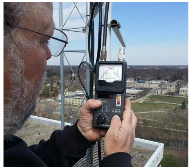
Steve, W8TER using an antenna analyzer
